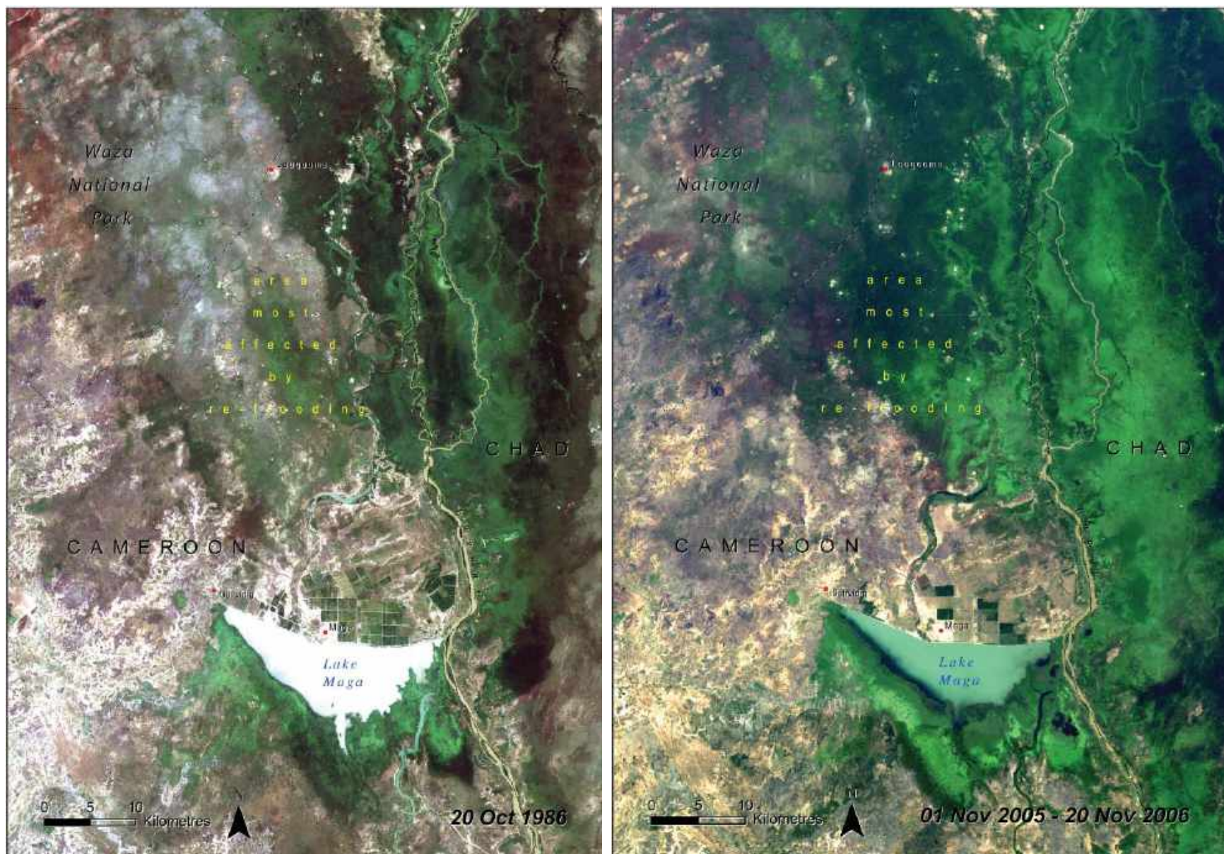
Figure 2.4.10: Damming of the Logone River in the 1970s coinciding with a period of drought reduced overbank flooding and disrupted local livelihoods on the Waza Logone Floodplain. Managed releases from the dam beginning in the 1990s restored some of the natural flooding, bringing improved grazing and return of other valuable ecosystem functions.
