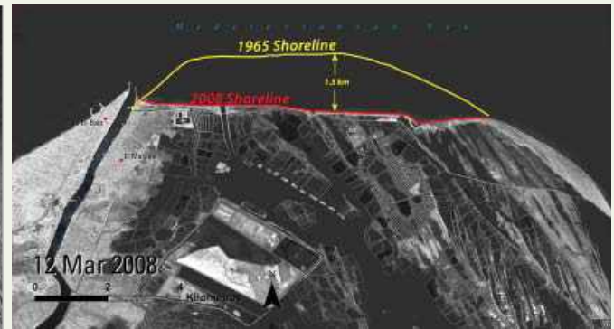
Damietta Promontory, formed by one of the two principle outlets of the Nile River, eroded 1.5 km between 1965 (yellow line) and 2008 (red line)
