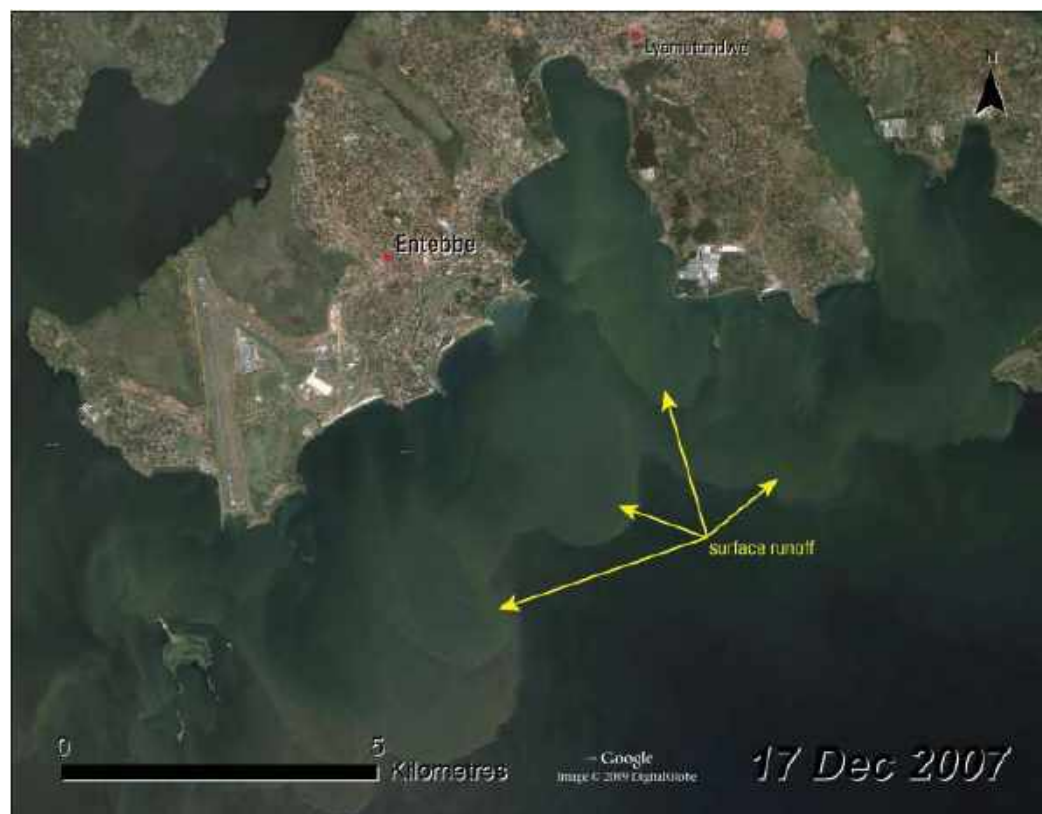
Figure 2.8.15: Surface runoff from the Entebbe area south of Kampala can be seen as greenish clouds expanding out into the water. Heavy runoff of domestic, industrial and agricultural waste as well as eroded soil is degrading the water quality of Lake Victoria
