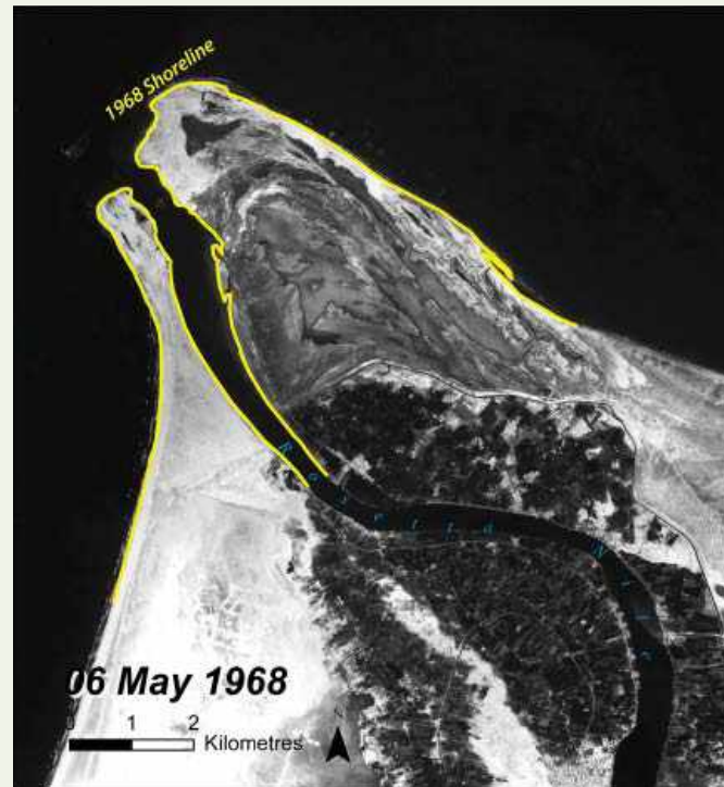
Rosetta Promontory lost over 3 km to erosion between 1968 (left image, yellow line) and 2009 (right image, red line)
